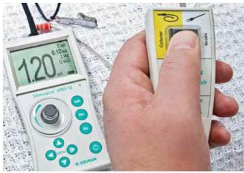
Change stimulation current from needle to catheter with the simple flick of a switch
